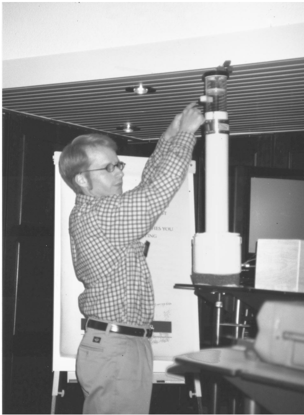
FIG. 2. Matthew Poese demonstrating a small, regenerator-based, thermoacoustic refrigerator.
